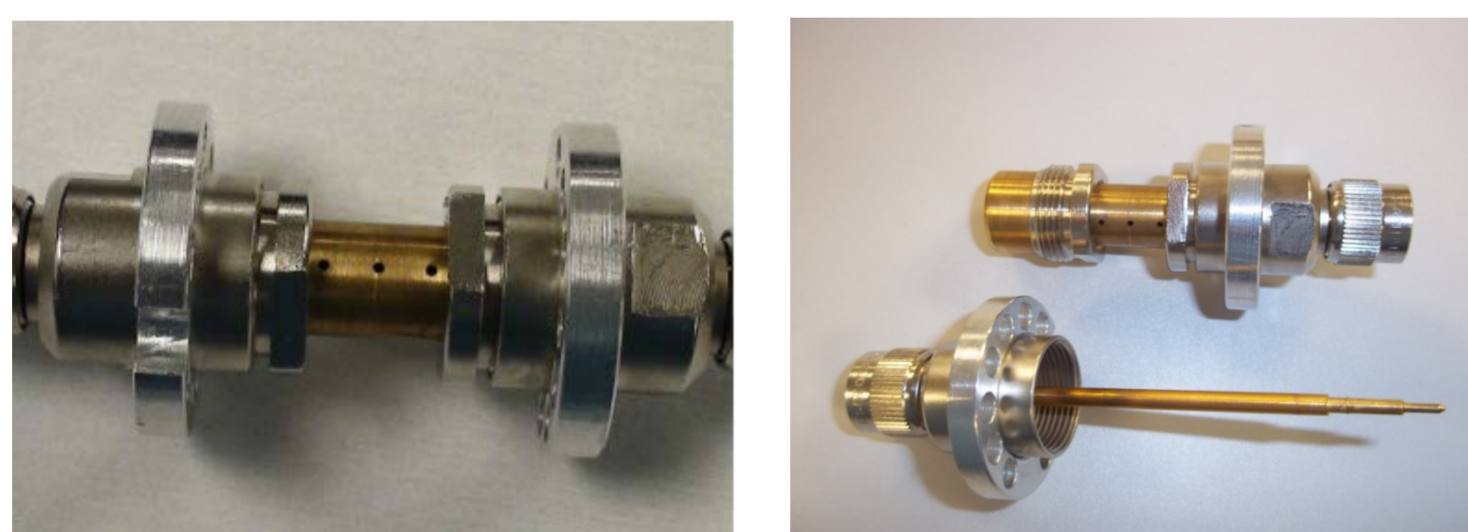
Fig. 1. Picture of the coaxial sample assembled (left) and disassembled (right).
